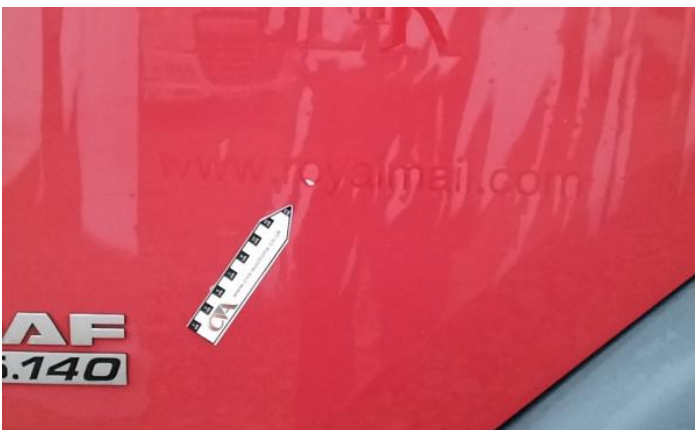
5: Wing nsf Scratched Over 25mm Thru Paint
