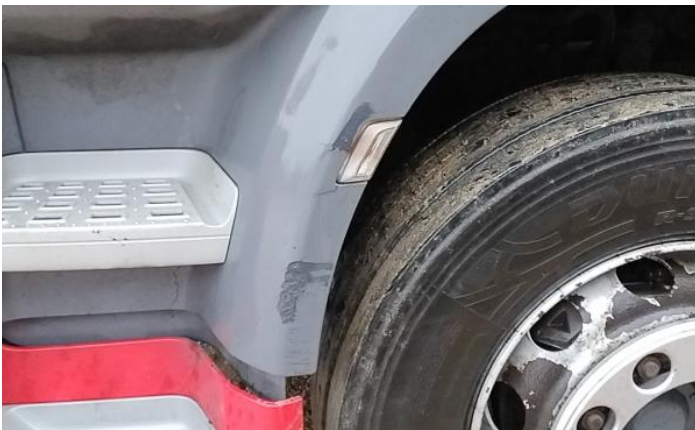
5: Fog Lamp Surround ns Scratched (Painted) Over 25mm Not Thru Paint
