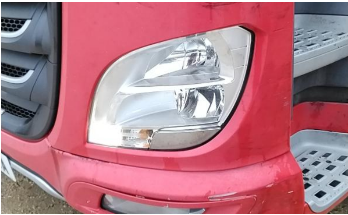
3: Bumper Front Dented With Paint Damage
